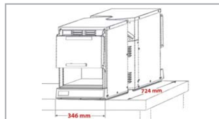
Two units fit back-to-back on a 724 mm (28 1/2") shelf in a 346 mm (13 3/8") space
